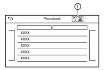
When a cellular phone is connected through the Bluetooth® wireless connection, indicators ① for phone and text messaging are displayed on the upper display.
