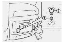
Commercially available headphones can also be used by connecting them to the headphone jacks ① located at the rear of the center console box.
