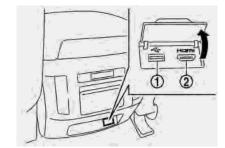
USB connection port 1 and HDMI port 2 are located at the rear of the center console box.
